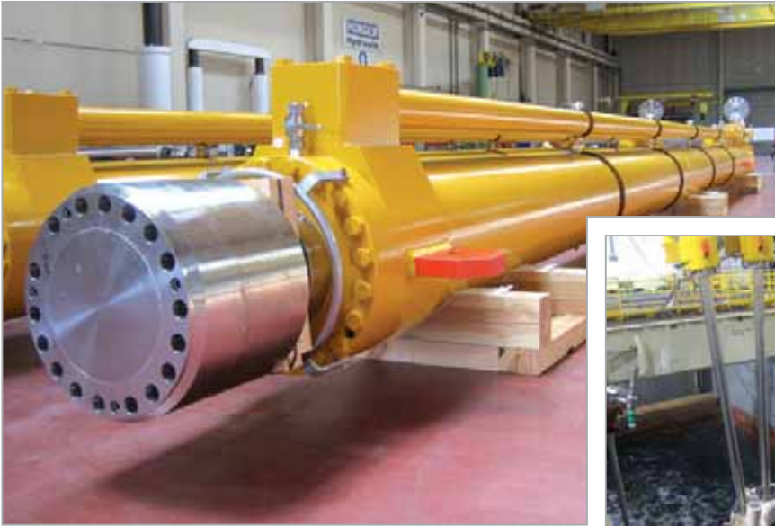
N- 直线张紧器缸 N- line tensioner cylinder
