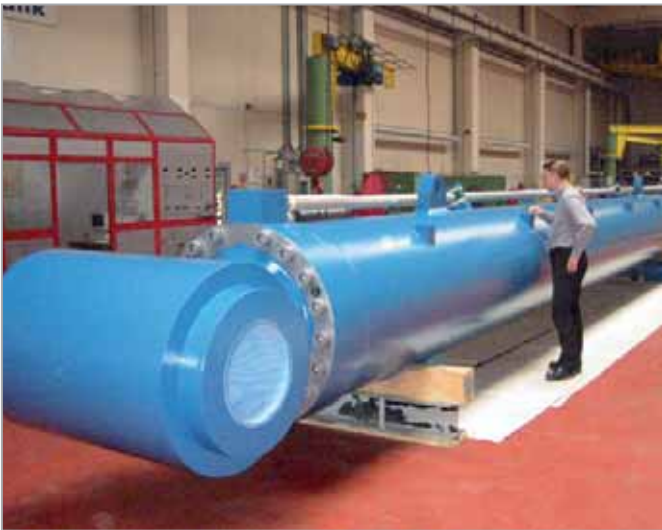
打桩船缸, 活塞直径900mm Piling barge cylinder with 900 mm piston diameter
