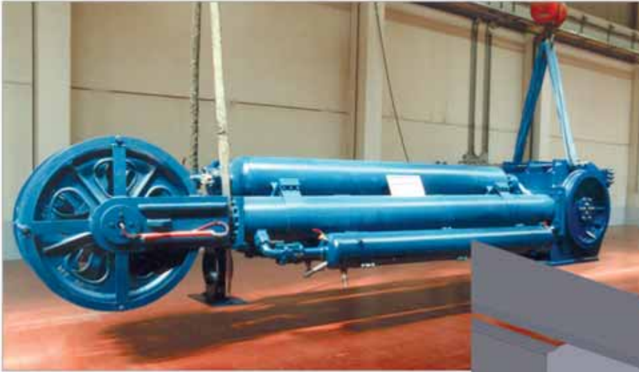
钢丝绳直线张紧器缸, 装有蓄能器和滚轮 Wire line tensioner cylinder with mounted accumulators and rolls
