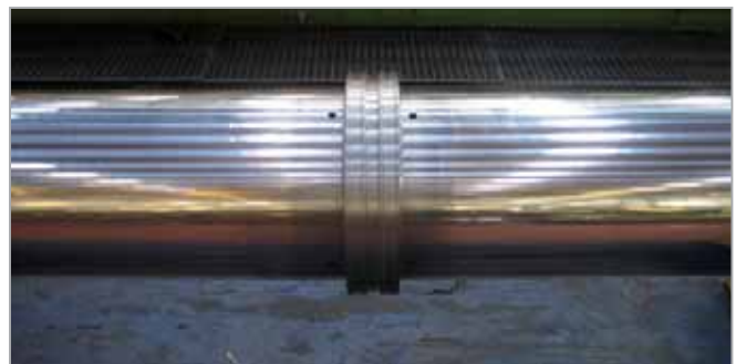
带有同轴活塞的双活塞杆, Ultraplate镀层和通过活塞杆供油 Double piston rod with centred piston, Ultraplate coating and oil feeding through the rod
